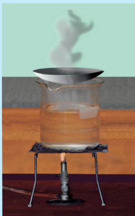
Figure 1.8 Experimental set-up for the determination of the solubility.
